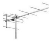
For VHF reception the Stellar model 30-2475 is not a bad choice for local reception. The length is 60.5", and it weighs 2 pounds. It claims between 9 to 12dB gain of a signal on channels 7 to 13. They are available from various locations, including MCM Electronics in Ohio. This antenna is designed for local reception. If you want a further reach it's best to step up to the 30-2476 which has more gain.
